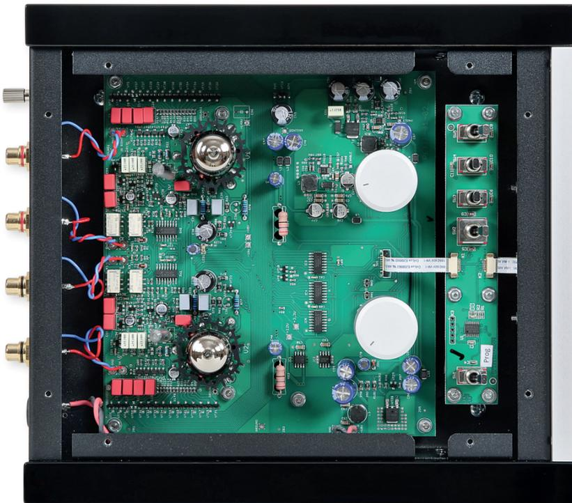
**RIGHT:** Powered by an outboard 18V DC PSU, the E-Glo Petit combines a discrete, low-noise J-FET front-end [near left] with a two-stage 12AX7 triode-based RIAA preamp [left]. Gain and loading options are switched by logic [centre]
